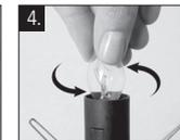
4. Twist the bulb in counterclockwise and pull the bulb in the direction of arrow. Do not insert any instrument in the holder.
