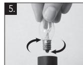
5. Take the new bulb, insert in the holder and twist it in the clockwise until it stops twisting further.
