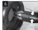
6. Press both hands of the spring to insert the bulb assembly inside the lamp.
